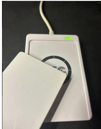
Figure 31: nfc card held to reader to receive data
